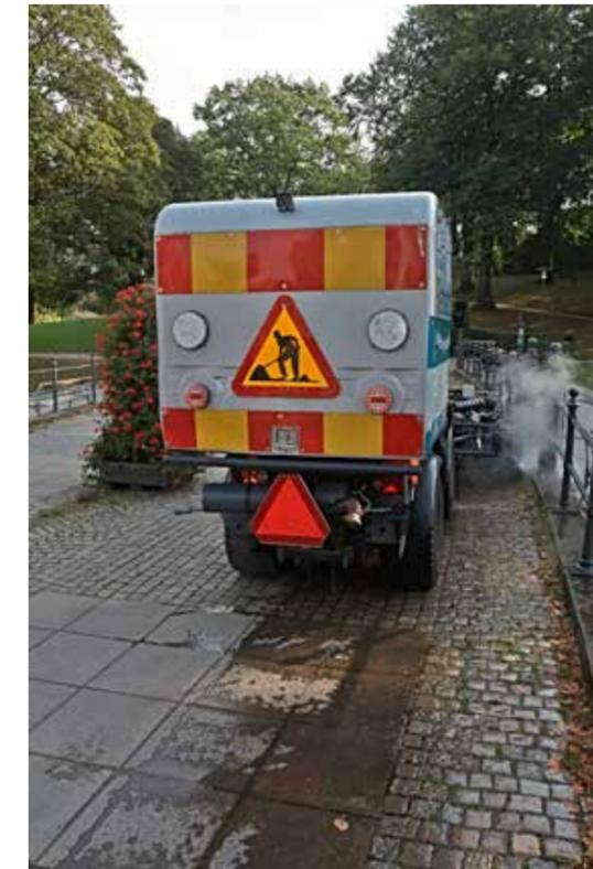
Sensors on deck control water spray levels - note how paving slabs with no weed growth detected have remained dry.
