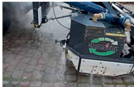
Close up of deck in operation show how hot water is targeted to where weeds grow. Water pressure is not enough to damage joints between fashionable block paving in downtown areas.
